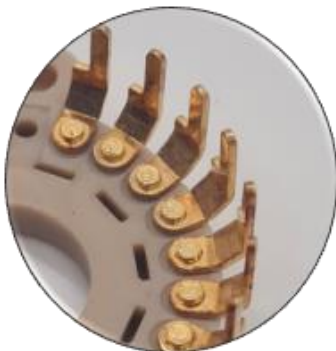
Hot riveting of contacts
